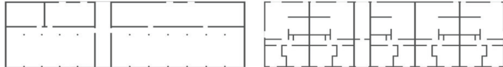
Open Front, Tuck-under Building: Weak with torsion due to earthquake loads in the long direction
