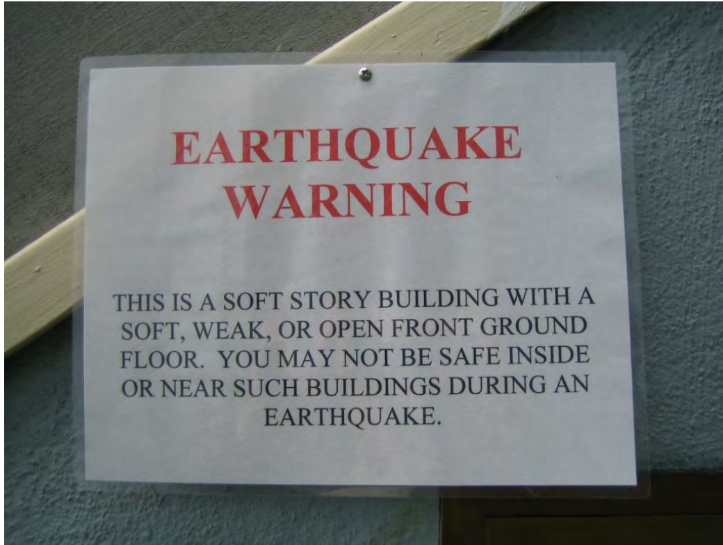
Figure 4: Photo of the warning sign mandated to be posted on buildings on the City of Berkeley's Suspected Earthquake Hazard Building List (Photo: S. Rabinovici, 2011).
